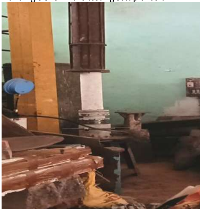
Fig 4 Testing setup for concrete column
