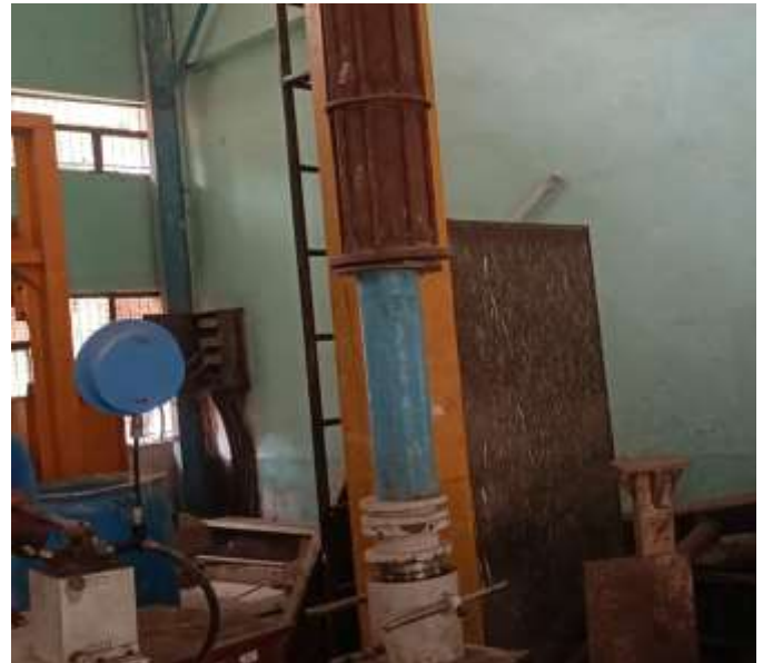
Fig 5 Testing setup of Strengthened column
